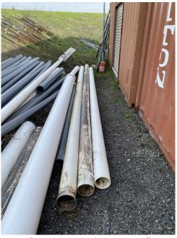
Pipes that go into Weirs ~ 30 - 40 lbs. (two – person lifts)
